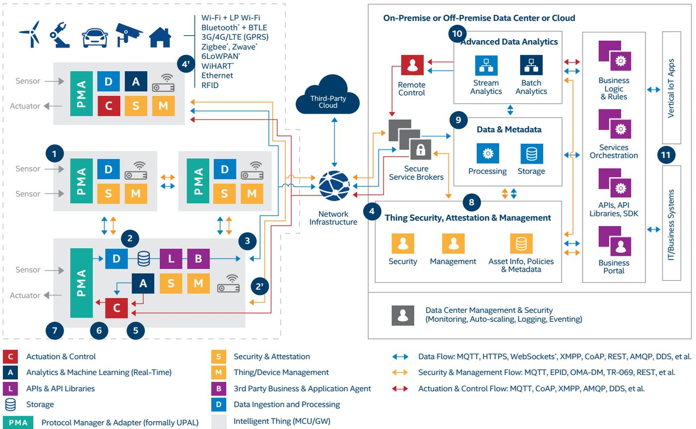
Figure 3. Data Flow for Devices without Native Internet Connectivity
