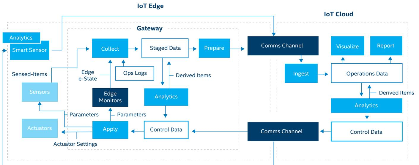
Figure 6. Data Layer Supports Distributed Analytics and Control
